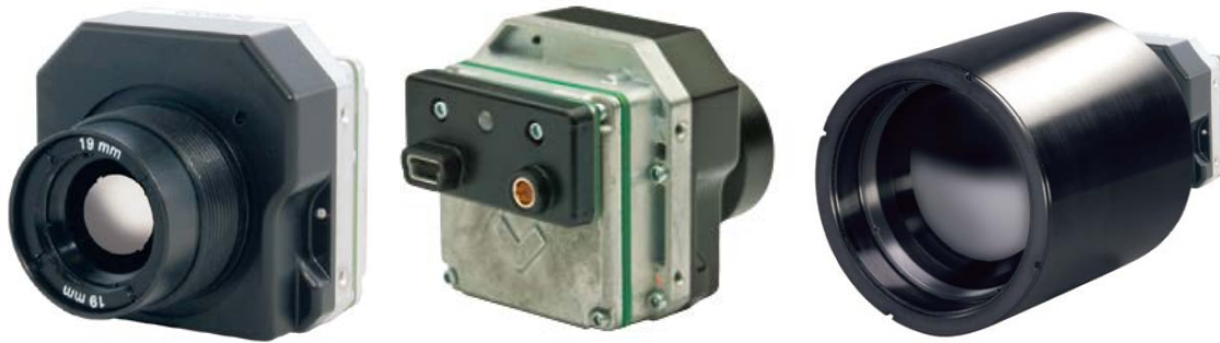
Figure 3. (left) Science payload is based on the FLIR Tau2 640 thermal imager. The imager is 4cm per side. (middle) Rear panel with USB connector interface board. (right) Imager with 100mm focal length lens as configured for our science payload.
