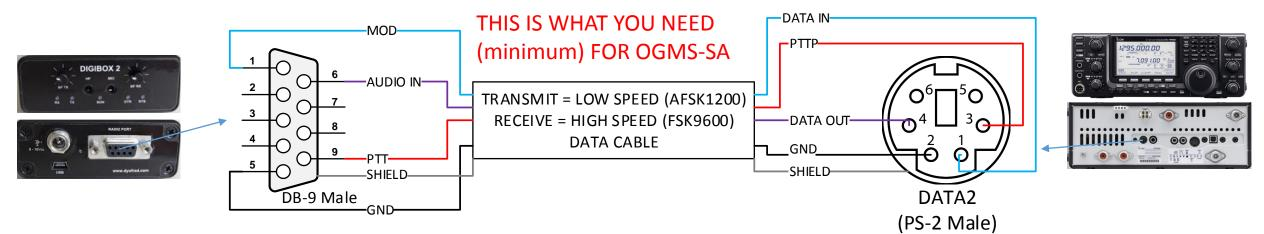
NOTE: In order to test this connection you need an FSK9600 Transmit reference signal. CANNOT use this cable with local APRS transmissions for testing.
